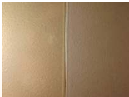
Img. 6.3.5. Color-deviation at dormant caused by two different shades in the oven
