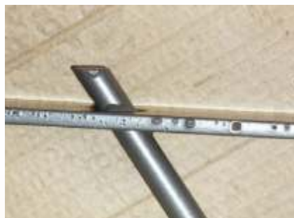
Img. 2.4.2. Bubbles caused by corrosion after pretreatment
