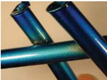
Img. 6.3.1. False position caused by incompatibility of the flux
