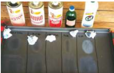
Img. 6.2.1. Greying caused by cleaning compounds
