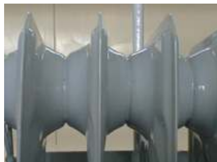
Img. 1.5.2. Rip up caused by poor metal-production
