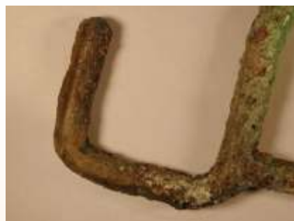
Img. 1.2.2. No earthing at multi coated hooks
