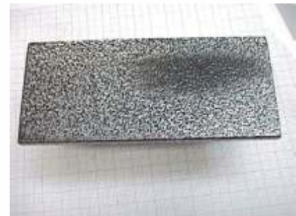
Img. 4.1.3. Metal particles oxidize at the cleaning
