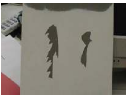
Img. 5.3.1. Poor adhesion caused by direct heated gas oven
