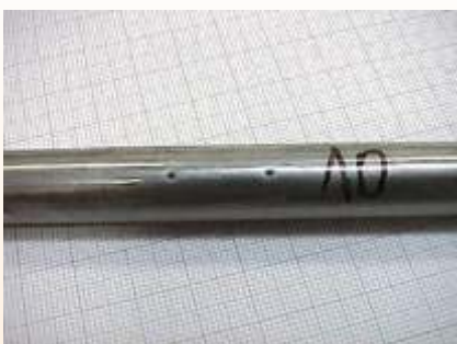
Img. 2.2.1. Crater caused by oil in the compressed air
