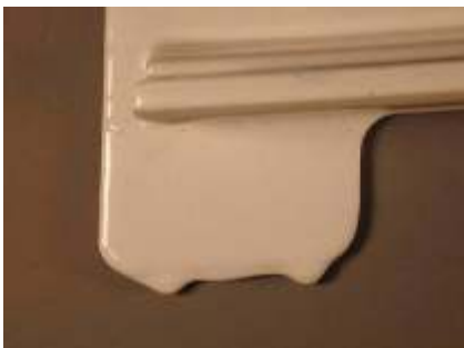
Img. 2.5.1. Drop formation caused by a too high film thickness
