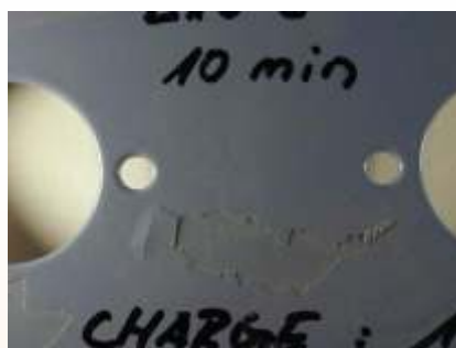
Img. 5.3.2. No adhesion of the top coat caused by directed heated gas oven
