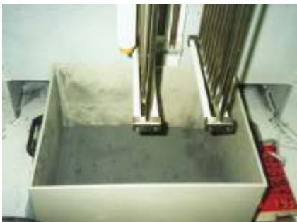
Img. 1.1.1. Fluidization - the powder has to flow like water
