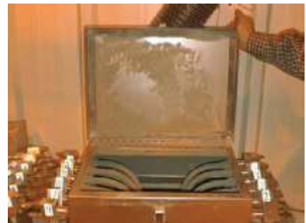
Img. 1.1.3. Poor fluidization - too much powder
