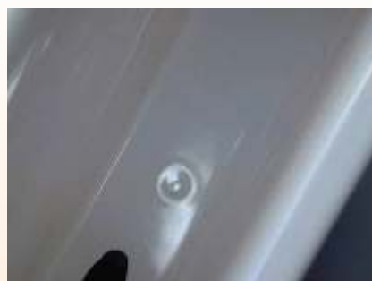
Img. 2.2.2. Crater caused by oil residue
